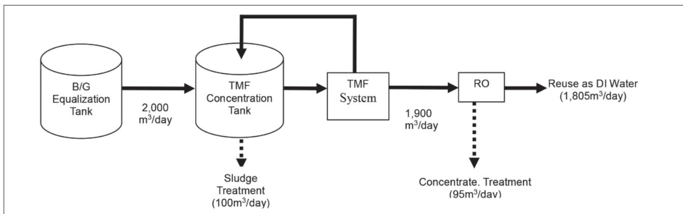
Schematic of the tubular membrane filtration system process
